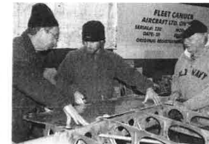
Canuck wing leading edge skinning: Bill Butler, Darren Hardwick, Ralph Rowe.
